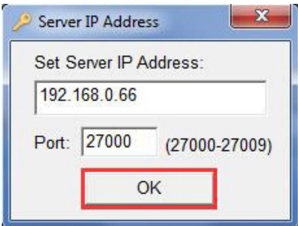
Click OK button to activate GstarCAD. With this client activation method, when you close GstarCAD 2016 software, the license will be returned to server automatically.
