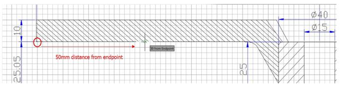
And within Object Snap tab, you can find a new added option called Divide Segments. This option allows snap the divided segment points of objects like line, arc, spline, pline, ellipse arc, mline and any
