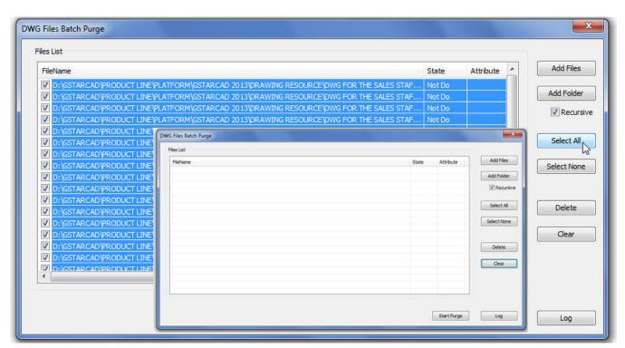
**Start Purge**: Starts purging the selected DWG file list and it shows a status bar during the execution. After purging, GstarCAD will generate a notepad file where you can see the purge details.
