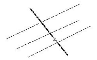
3. Choose the occluded (to be disconnected) line and what you selected will be cut off automatically as shown below.
