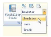
Click the "Invisibility" button in the Visibility tool panel, select truck and car drawings, then make them invisible in the "roadster" state, as shown in the following picture, after selecting, press enter to confirm. For the state of "Car" and "Truck", set them in the same way.
