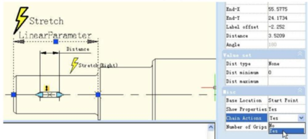
Add Stretch Leftwards action for keyway as the following picture shows. Special Notes: Do elect "Distance" to linear parameter to stretch leftwards operation objects set. This is a necessary procedure of chain operation.
