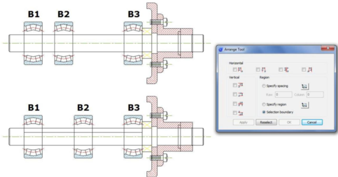
Another example, we can apply this tool for arrange the part numbers distribution over the leader lines. Notice that the objects to be selected are Mtext and will be distributed according to the top object level as a reference. After started the command, a prompt message will display > Please select the object to arrange:
