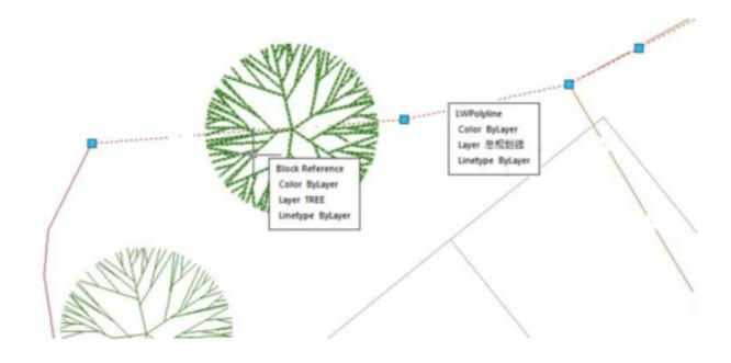
After starting LAYOUTBYPATH command, follow the steps below: 1. Please select the object to array: Select the object (block)
