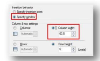
**Rows**: Specifies the number of rows. When the Specify Window option is selected and you specify a row height, the Automatic option is selected, and the number of rows is controlled by the height of the table. A table style with a title row and a header row has a minimum of three rows. The minimum row height is one line. If a table style containing a starting table has been specified, then you can choose the number of additional data rows you would like added to that starting table.
