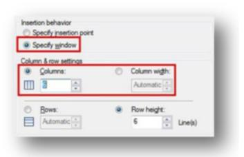
**Column Width**: Specifies the width of the columns. When the Specify Window option is selected and you specify the number of columns, the Auto option is selected, and the column width is controlled by the width of the table. The minimum column width is one character.
