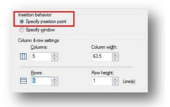
**Specify Window**: Specifies a size and a location for the table. You can use the pointing device or enter coordinate values at the Command prompt. When this option is selected, the number of columns and rows and the column width and row height depend on the size of the window and the column and row settings.
