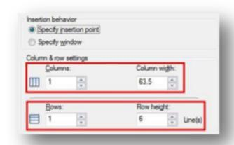
**Columns**: Specifies the number of columns. When the Specify Window option is selected and you specify a column width, the Automatic option is selected, and the number of columns is controlled by the width of the table. If a table style containing a starting table has been specified, then you can choose the number of additional columns you would like added to that starting table.
