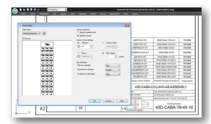
**Table Style**: Choose a table style from within the current drawing from which to create a table. You can create a new table style by clicking the button next to the drop-down list.
