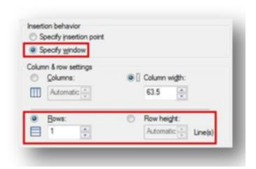
**Row Height**: Specifies the height of the rows in number of lines. The height of a line is based on the text height and the cell margin, which are both set in the table style. When the Specify Window option is selected and you specify the number of rows, the Auto option is selected, and the row height is controlled by the height of the table.
