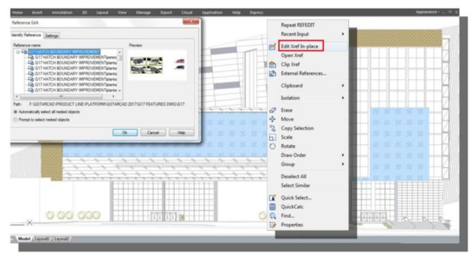
The objects that you select from the selected xref or block are temporarily extracted and made available for editing in the current drawing. The set of extracted objects is called the working set, which can be modified and then saved back to update the xref or block definition.
