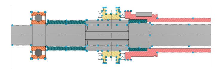
It is possible to directly draw symmetrical shapes with SymmetricDraw tool. When drawing the first half you get another half automatically.
