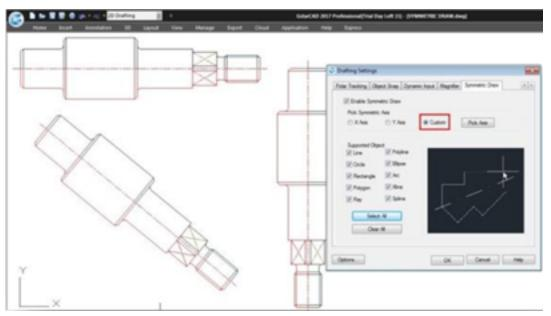
**Pick Symmetric Axis**: At status bar, besides Symmetric Draw button is located another button called Pick Symmetric Axis. The functionality of this button is as same as Custom and Pick Axis options.
