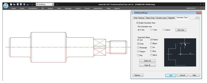
Users can easily switch on/off this tool by clicking the Symmetric Draw button on the status bar. By the way, Symmetric Draw tool supports all the drawing commands of GstarCAD.
