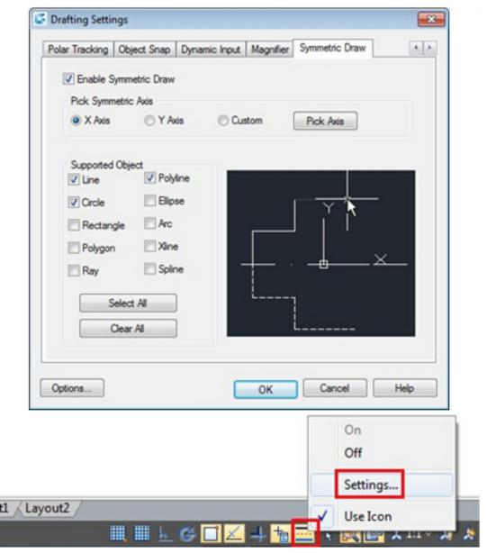
**Enable Symmetric Draw**: Enables the symmetric draw tool if is checked.
