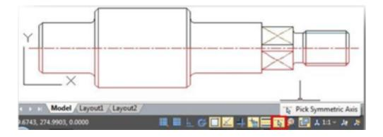
Technical Demo - Symmetric Draw is an innovative tool to directly draw symmetrical shapes. When drawing the first half you get another half automatically.
