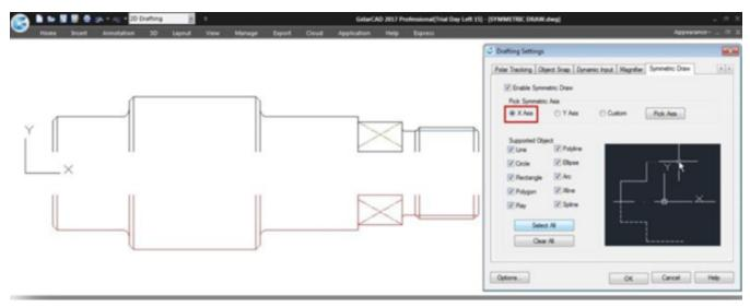
**Y** Axis option: The objects drawn will take the Y coordinate system as invisible axis line. The effect of Y Axis is mirroring the drawn objects right or left side according to Y coordinate system origin location.
