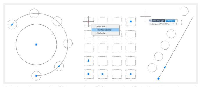
Each element in an array is called array project, which can contain multiple objects. You can also specify blocks as source objects for arrays. If you choose the path array, you also need a straight line, a polyline, a three-dimensional polyline, a spline, a helix, an arc, a circle, or an ellipse to use as a path. For different array types, the Ribbon panel provides different parameter setting options.
