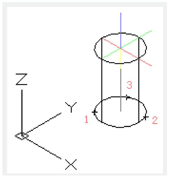
**2p**: Specify the cylinder height by 2 points, the distance of 2 points determines cylinder height. **Axis endpoint**: Specify the endpoint of cylinder axis. The axis endpoint could be center point of top plane; as well it could be any place in 3D space. The axis endpoint defines the length and direction of cylinder.
