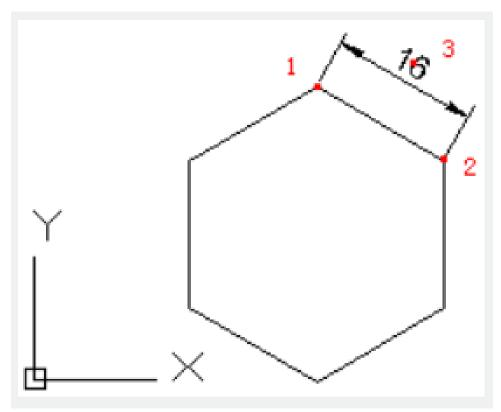
**Extension line origin** : Specify the first point of dimension extension line and then specify the second point of dimension extension line.
