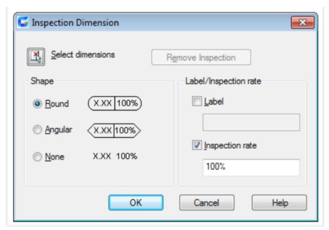
In Inspection Dimension dialog box, users could add or remove inspection dimension of existing dimensions. The inspection dimension could effectively express inspection rate and keep dimension and tolerance within specified range
