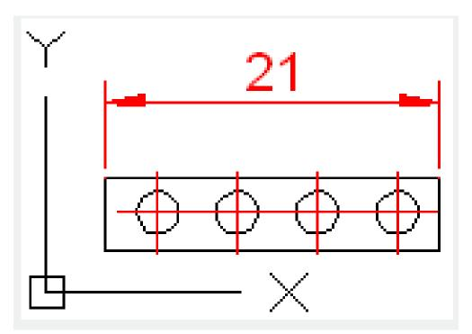
**Angle**: Change the angle of dimension text. The angle is measured from the X axis of UCS and the text rotation center keeps still. If the angle is 0, the text will be placed in default position. Moving dimension text or regenerating it, the direction of text will not be changed.
