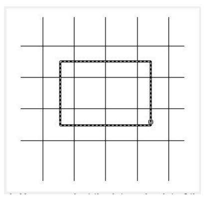
4. Here we select the internal point of the rectangle, you will see that the internal lines of the rectangle are trimmed.
