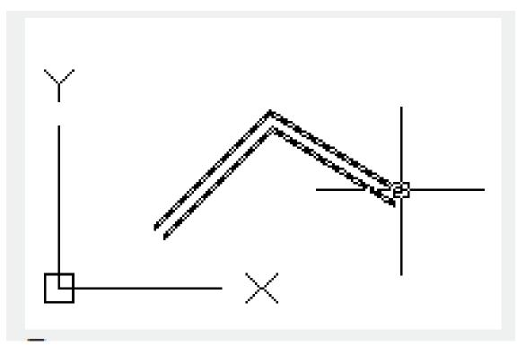
Zero: Place the cross cursor to origin and draw multiple lines. The "elements" options of the MLSTYLE command could specify the offset to 0.0.
