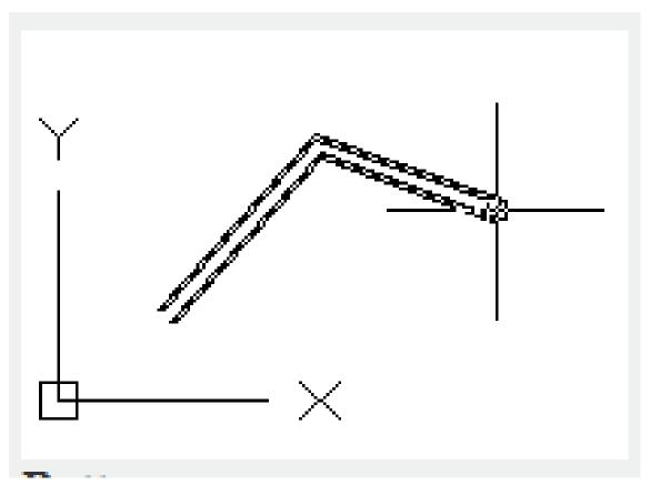
**Bottom**: Draw multiple lines above the cross cursor. The line with maximum negative offset appears at the specified point.
