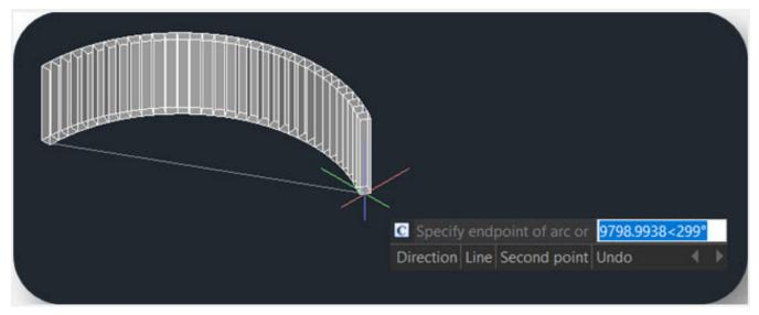
If you type "**Arc**", it can give you 3 options (Close, Direction, Line), you can draw the arc by 2 points or enter "Direction" to draw the arc by tangency direction.
