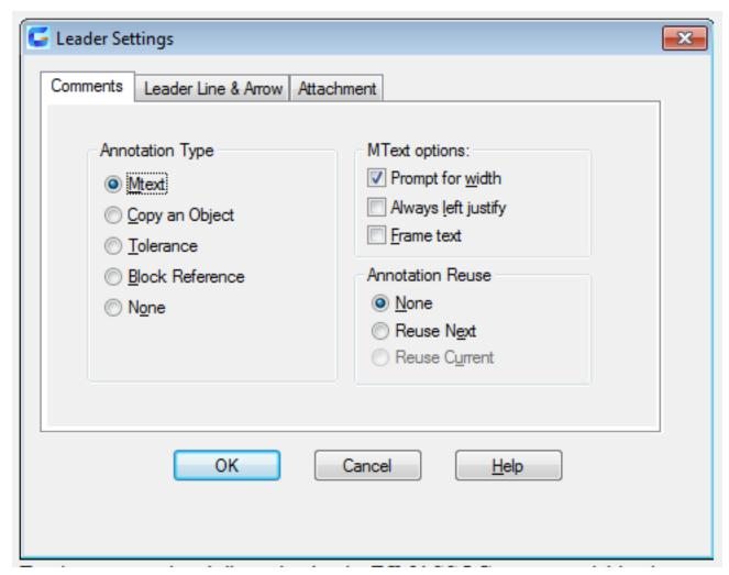
Turning on associated dimension by the DIMASSOC system variable, the start point of leader will be associated with the objects position. If repositioning the objects, the leader will be stretched and the arrows are attached to the objects still, but the text and position of properties control box will not be changed.
