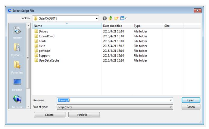
The script file is one kind of text file with ".scr" extension. Each line in script files contains commands that could be executed under command prompts. Users could input the script file name in the "Select Script File" dialog box to run it. If the FILEDIA system variable is specified to 0, the SCRIPT command will display command prompts.
