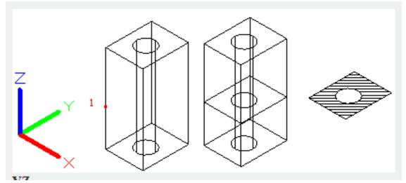
**YZ** : Align the section plane to the YZ plane of current UCS.
