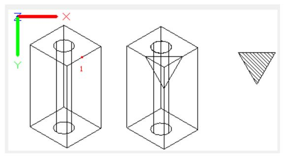
**XY**: Align the section plane to the XY plane of current UCS.
