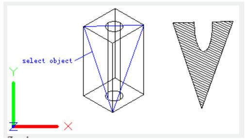
**Z** axis : Define a section plane by two points; one point goes through section plane and another point is on the Z axis (normal).
