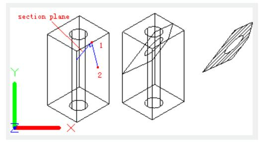
Specify a point on the section plane:Specify one point on the plane.Specify a point on the Z-axis (normal) of the plane:Specify one point to define a plane that is perpendicular with Z-axis.
