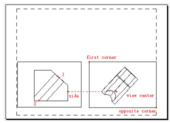
Create a section plane by two points in original viewport. Specify the side of view by selecting one point. Users could scale viewport by inputting view scale, the default value is 1, the scale factor is equal to zoom 1.0×p. Users could define the view center under the prompt of "specify view center". Press ENTER to accept the default scale, the vertical line appears to guide locating the view center; otherwise, users could place the section view at any position.
