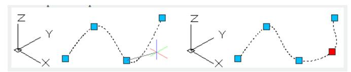
After selecting a fit point on the spline, please specify a new fit point to add to it along the spline direction.
