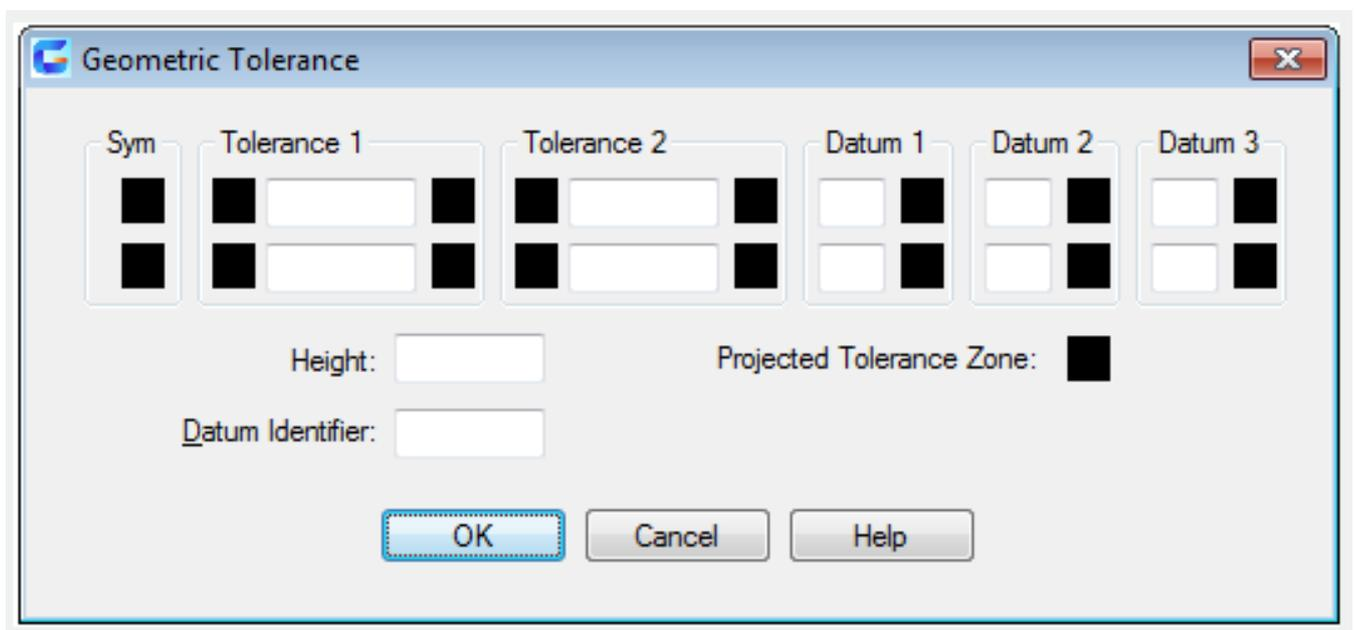
The geometric tolerance is the allowable deviation of shape, profile, direction, position and beat. The feature control box could be created by the TOLERANCE or LEADER or QLEADER command with leader.
