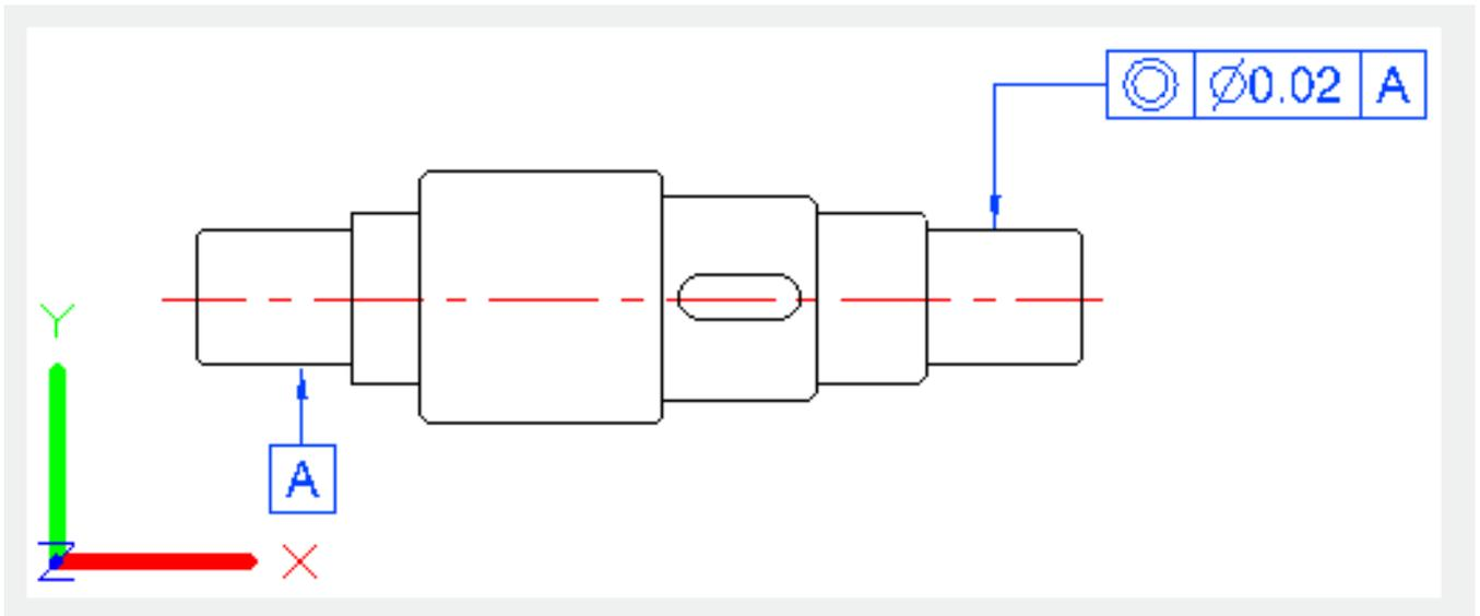
The TOLERANCE dialog box is used to specify the symbols and values for a feature control frame.
