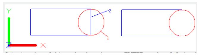
Select boundary of object to be trimmed or press ENTER to select all displayed objects as potential boundaries. The TRIM command will project the boundary and objects to be trimmed into XY plane of current UCS.
