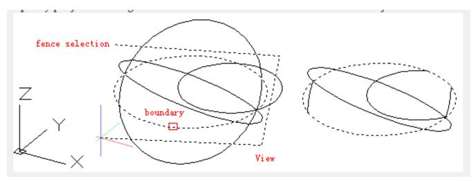
Edge: Determine to trim the object at the intersection in 3D space or on its extended edge.
