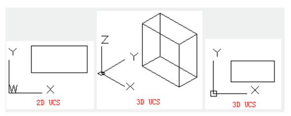
**3D:** if the current UCS is the same as WCS, looking down the UCS (the positive direction of Z axis), the origin in XY plane displays as a box; looking up the UCS, the box disappears.
