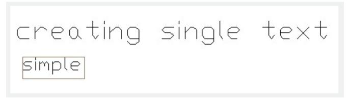
When you create single-line text, you can use current text style or specify another text style, you can specify the start point, height, rotation angle and justify of text.
