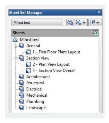
In Sheet Set Manager, a sheet set is an organized collection of sheets from several drawing files and each sheet in a sheet set is a layout in a drawing file.
