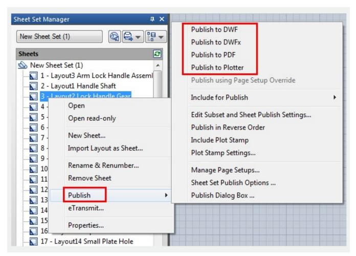
This method is used to plot and publish when the page setup is set per layout. The drawback to using this option is if someone plots one of the sheets using the plot command and saved the setup to the layout, the layout will not publish properly. Sheet set can also be packaged and shared through e-transmit. Publishing using Publish dialog box may not be as fast as Publishing directly to the plotter/file, but there is less of a chance the document will come out wrong.
