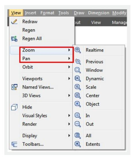
You can change the magnification of a view by zooming in and out. ZOOM does not change the absolute size of objects in the drawing.
