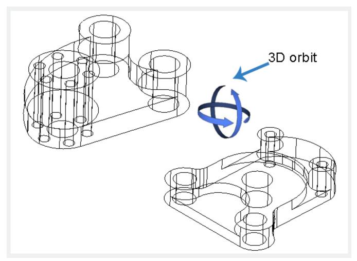
When you activate <u>3D navigation</u> you can <u>PAN</u> and <u>ZOOM</u> at the same time. During a 3D navigation operation, it is not allowed to manage or edit entities in the drawing
