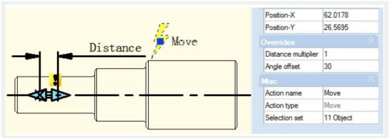
Select the Dynamic Block and then move the right side grip. You will find it can only move in the direction of 30° as it is shown in the follow picture. The direction of action can change according to the Angle Offset.
