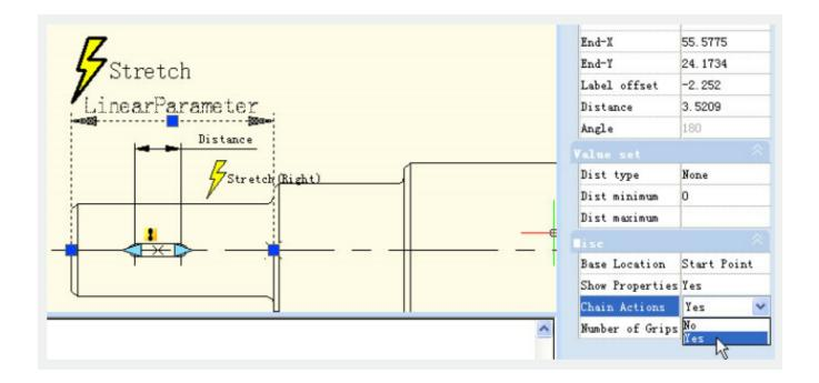
Add the Stretch Leftwards action for keyway as the following picture shows. Special Note: Do elect "Distance" for the linear parameter to stretch leftwards the operation objects set. This is a necessary procedure of the chain operation.
