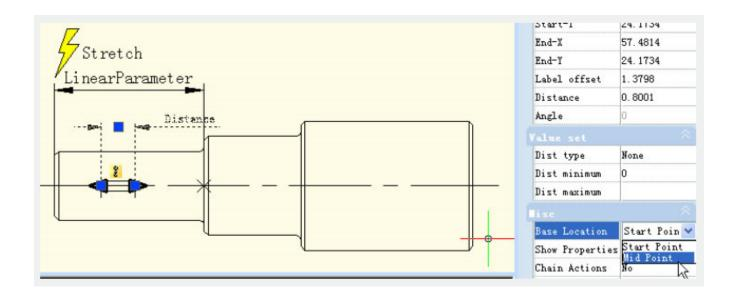
3.Add the stretch rightwards action for the keyway
