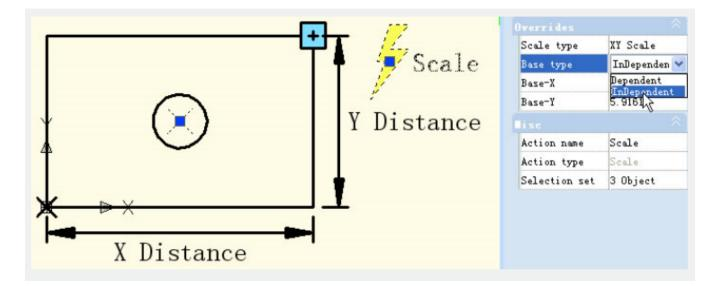
Specify new base: Single click the right input box of "Base-X" and "Base-Y", you can manually input the
