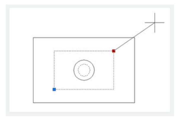
After modifying Base type and position, the scale center of the dynamic block changes from the XY Parameter base point to the new specified base point (center of the circle).
