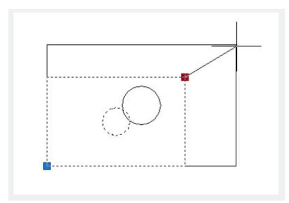
It is easy to find that both the circle and the rectangle scale by the base point of the XY Parameter.
