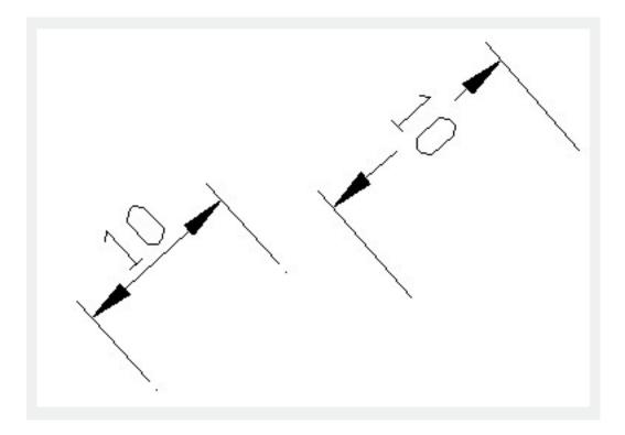
If you want to rotate or replace a dimension text, You need to specify the change first, for example, rotating the text to be at 45 degree.
