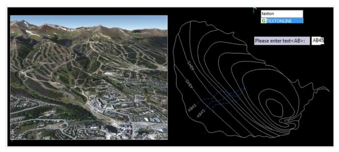
Text on line also offers a couple of options to modify the written text: Please pick the curve Modify Text (X) / Modify Type (T) / Modify Method (M) / Modify Text Height (h):
