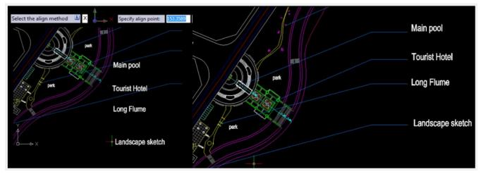
And finally, if we choose the Two points (P) alignment method and then specify two points to align the texts in the correct location (start and end point of Leader). The result is as follows:
