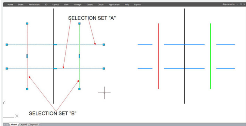
Break objects touching selected objects: With gap value of 10 for each break point.
