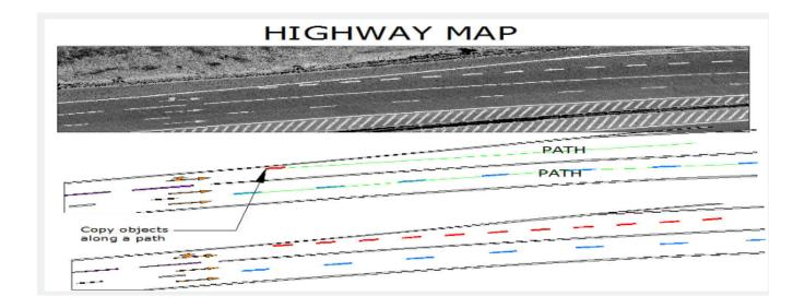
After starting the command Layoutbypath a message will be displayed in the command line>Please select the object to array:
