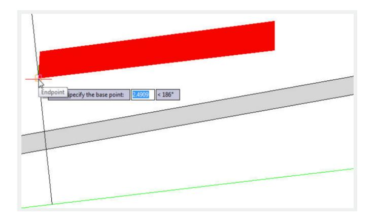
After selecting the base point of the object, a prompt message will be displayed: Specify the object's direction along the curve<Y axis of WCS>:
