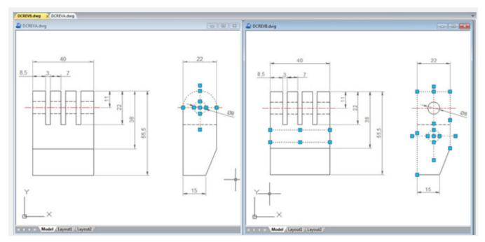
Drawing compare can make comparisons between two similar drawings (Old DWG and New DWG) and generate them as separate files. After pressing COMPARE button within Compare Dwg dialog box, the program will generate and open \_old and \_new.dwg files, where you can see the differences between drawings.
