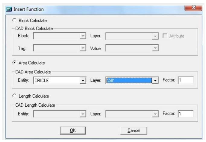
11.Use the same operation to insert the rectangle area calculating function, as shown below.
