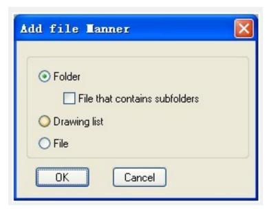
Folder: This option will add all the DWG files from the root directory to the arranged list, if you check "File that contains subfolders" option and all the DWG files from subfolders will be added to the arranged list.
